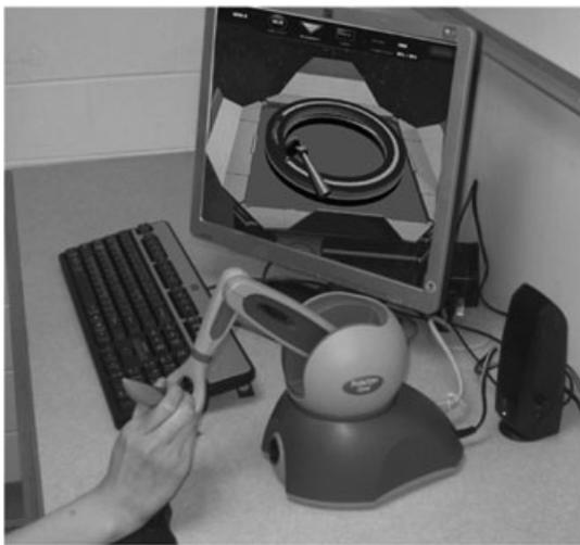
Figure 5. SensAble PHANTOM Omni<sup>®</sup> haptic device used for training
